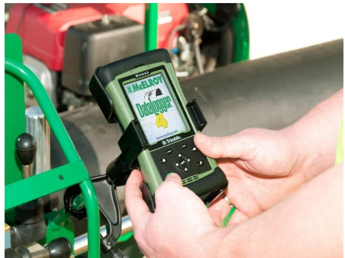
Datalogging technology brings accountability to a new level as owners and inspectors can monitor operator performance in real time from down the block or from across the continent.
