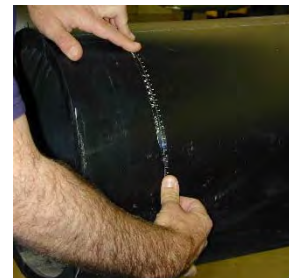
Figure IV-a - Measuring pipe diameter with Pi tape
