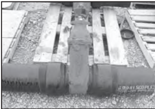
Figure 21 Ductile Iron Gate Valve with PE Ends
