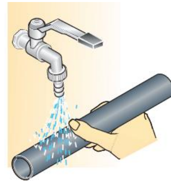
Figure X-b – Clean Pipe Ends
