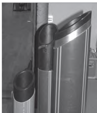
Figure 22 Protecting the PE Pipe from Shards
