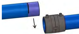
Figure X-h – Repair - Coupling Over Entire Pipe End
