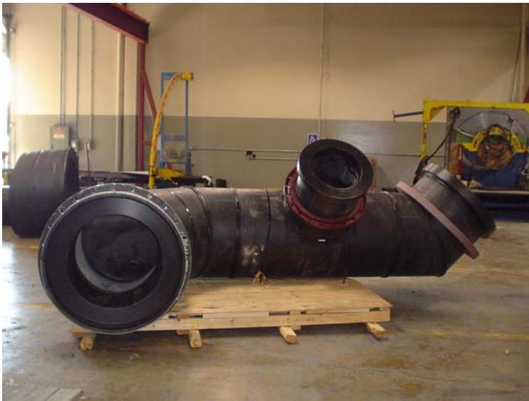
Figure 7 Fused Manifold Assembly with Flange Adapters And Back Up Rings
