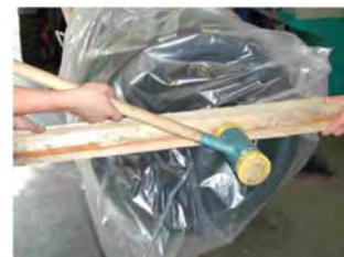
Figure X-g – Avoid Contamination During Installation
